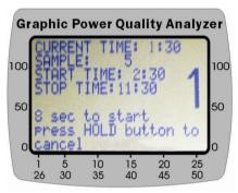
Users always have 8 seconds to cancel Datalogging by pressing the HOLD button for **about 2 seconds**. If users do not press HOLD/CANCEL button, the unit starts Datalogging, and **the LED next to the REC button starts blinking**.
