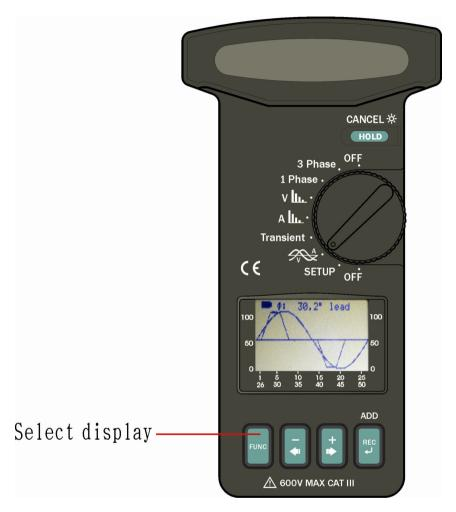
When users set the rotary switch at waveform position, the unit will display both voltage and current waveform with phase angle.
