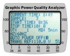
**TRANSIENT REFERENCE:** set the nominal voltage and threshold (%) for transient capture.
