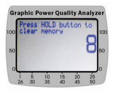
If users do not press the HOLD button in 8 seconds, the memory is not clear. This timer could avoid users accidentally clear the memory.
