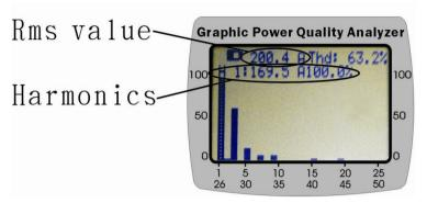
%THD-F: Total Harmonic Distortion with respect to Fundamental frequency
