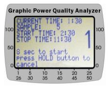
Users always have 8 seconds to cancel Datalogging by pressing the HOLD button for **about 2 seconds**. If users do not press HOLD/CANCEL button, the unit starts Datalogging, and **the LED next to the REC button starts blinking**.
