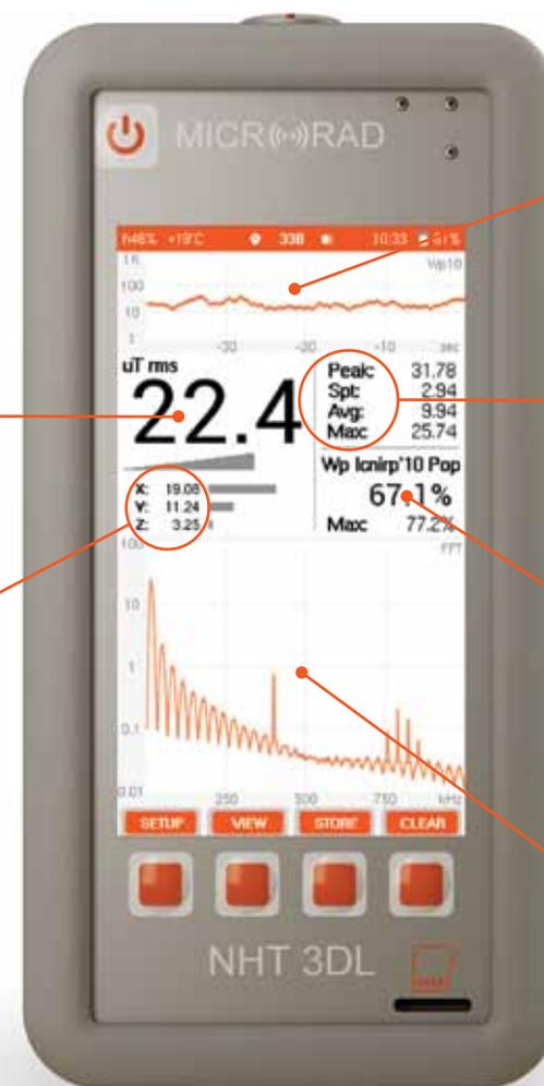
$$WP_{10} = \left| \sum_{i=1\text{Hz}}^{1\text{MHz}} \frac{A_i}{EL_i} \cos(2\pi f_i t + \theta_i + \varphi_i) \right| \leq 1$$
