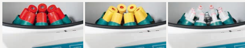
Angle rotor illustrated with different blood collection tubes
