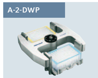
A-2-DWP 2-place deepwell plate rotor for plates up to 89 mm loading height. Max. speed 2,250 \times g (3,750 rpm).
