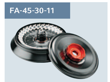
FA-45-30-11 30 x 1.5/2 mL micro tube rotor with aerosol-tight lid for safe centrifugation of hazardous samples. Max. speed 20,800 \times g (14,000 rpm).
