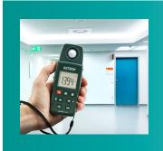
Measures light intensity up to 1860 Foot-candles (20,000 Lux) with resolution to 0.1 Fc/1Lux. Ideal for indoor lighting tests and for checking security and safety illumination in parking garages, night time ATM areas, stairwells, landings, and hallways.
