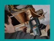
Light weight VideoScope includes a wired handset and 6mm diameter camera with 240° articulating tip for best viewing angle. Easy one-hand operation of the articulating camera tip facilitates viewing in obstructed areas where standard camera tips cannot access. Images and videos are viewed on the large high resolution color display or external monitors and can be stored in SD memory card (included) or a USB flash drive.
