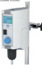
The **DLH** is a digital overhead stirrer for **medium viscosity** liquids.
