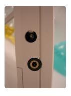
The built in DC socket allows the htV-M to be powered by the mains if used as a continuous data logger, so as to save the internal battery of the unit.
