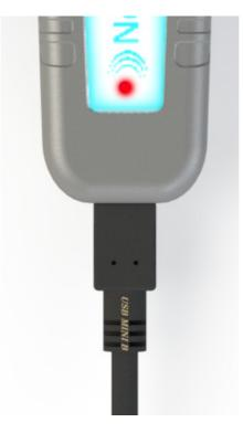
The actual time to fully charge a NoisePen will depend on the current capability of the USB source, but will typically be less than four hours for a fully discharged NoisePen.
