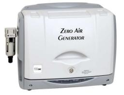
VICI DBS GC Zero Air Generators are designed to supply ultrapure hydrocarbon-free zero air for GC-FID applications. Catalytic oxidation technology eliminates hydrocarbons to <0.1ppm, resulting in a flat, stable baseline, increased sensitivity, and repeatable analysis.
