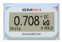
The GM08 Gaussmeter has been designed and manufactured by Hirst Magnetic Instruments Ltd. A company with more than 60 years experience in Magnetic Measurement. This experience together with our extensive knowledge of the magnetics market has enabled us to design an instrument incorporating all the measurement functions a user is likely to need. The GM08 is controlled via a simple menu and is supplied with a thin semi-flexible Tranverse Hall Probe or a rigid axial probe.
