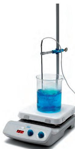
AREC.X with support rod and external probe
