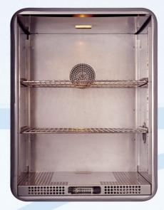
The right materials was chosen for the construction of the product to ensure maximum durability and reliability. The chamber is made of stainless steel that does not show any deformation although it is subjected to sudden temperature changes during operation. The outer body including the door is made of epoxy-polyster powder coated stainless steel to resist high humidity levels.
