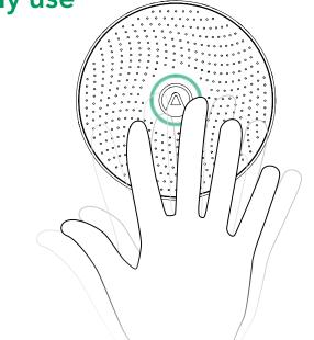
Wave in front of your detector and a light ring will glow for a few seconds to indicate your radon levels.
