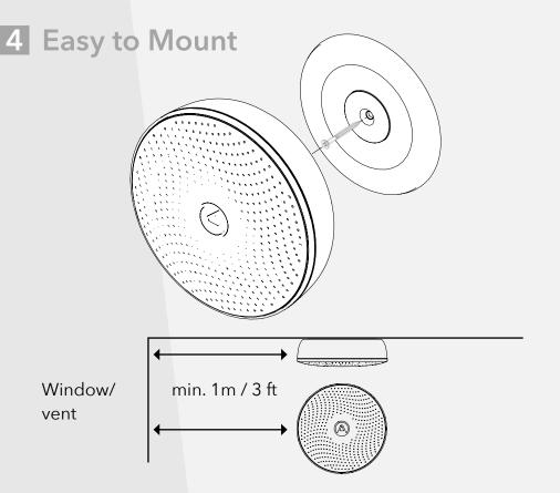
Fix the mounting bracket to the ceiling or wall. Make sure you use appropriate screws for your wall type. The screws included are intended for wood or concrete walls. Do not place it close to vents or windows. Minimum 1 meter / 3 feet distance.
