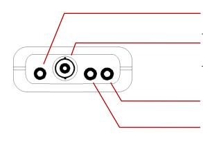
**interface:** connection for galv. Isolated interface adapter (accessory: GRS 3100, GRS3105 or USB3100)
