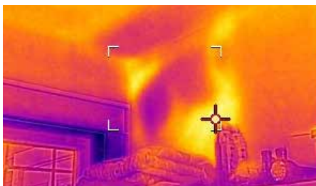
See temperature patterns showing insulation voids and other building issues
