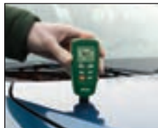
Measuring the thickness of automotive paint
