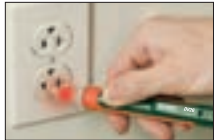
Flashing Red LED with audible beeper indicate presence of live wires.
